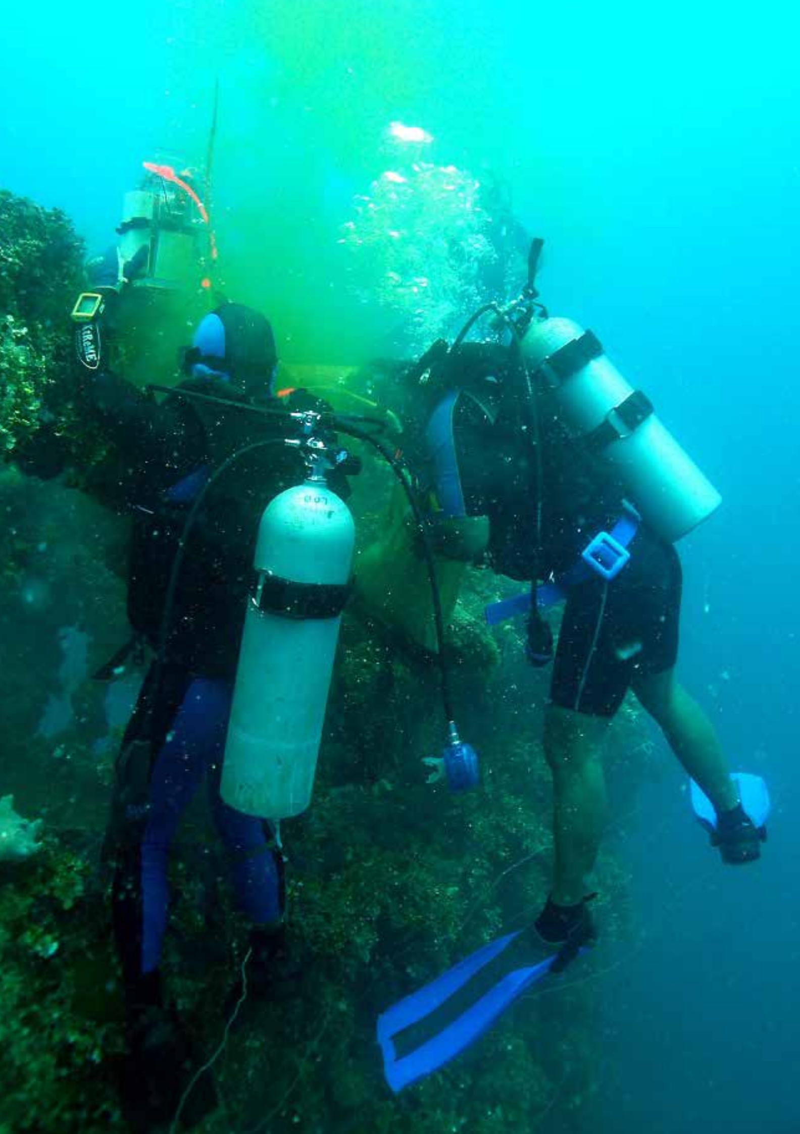
**Figure 5-11.** Taking corrosion measurements on the hull of *Kensho Maru*. This part of the vessel was in poor condition as can be seen by the corrosion plume that was produced by drilling into the hull. © Bill Jeffery, 2007
