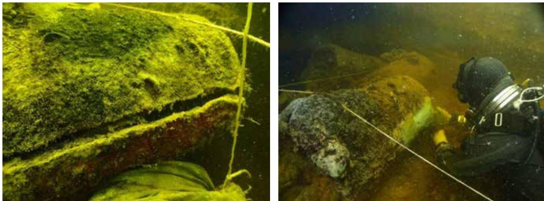
a. Crack along the welding seam
