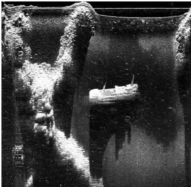
**Figure 5-7.** *Sapporo Maru* can be seen to the right of middle in this side scan sonar image. The vessel is sitting upright and intact with a slight list to starboard (right). The bow is to the left, forward and stern masts can be seen lying to starboard, and the start of the bridge is clearly evident about half way back along the vessel. The relief of the vessel has caused the seabed to the left of the vessel to be in shadow. Other seabed features (in white) are natural reef. ©Jeremy Green
