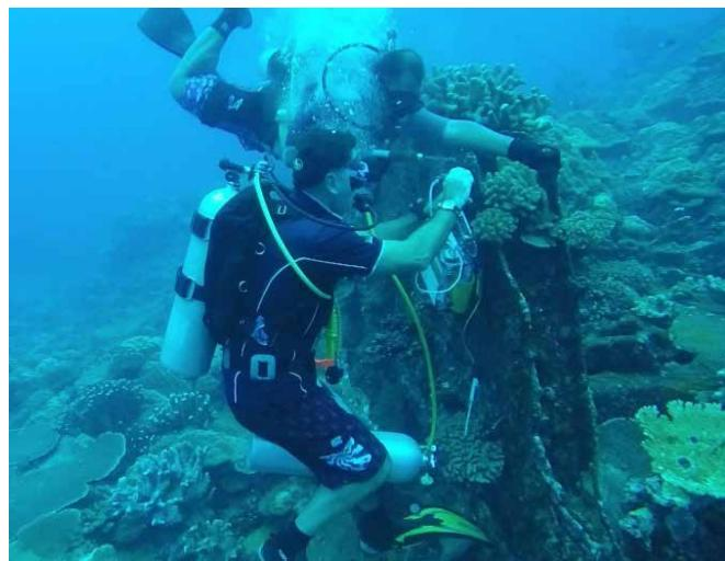
**Figure 6-7.** Divers conducting a corrosion survey on the remains of the *Nissei Maru* (1942) in Flying Fish Cove, Christmas Island. ©Wreck Check Inc
